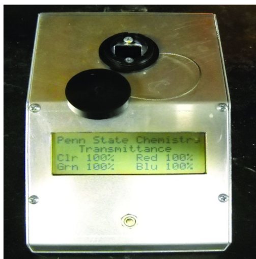
Figure 5. Student-made colorimeter was designed and built for <$50. (see color insert)
